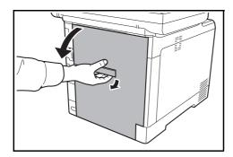
1 Pull up the rear cover lever and open the rear cover.
